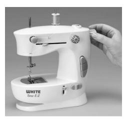
Rotate the handwheel to bring the needle to the highest position.
